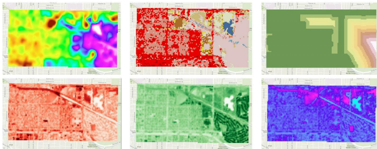
Figure 4: ArcGIS raster layers example clockwise from left: Land Surface Temperature; Land Cover Type; Distance to Nearest Road; Shortwave Infrared Reflectance; Near Infrared Reflectance; Infrared Reflectance
